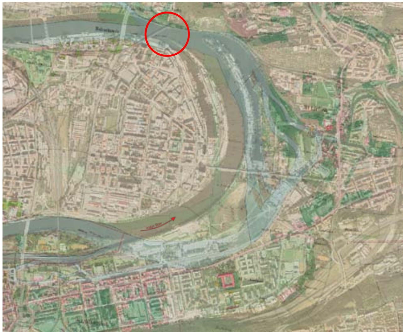
Fig.67.: Bottleneck. By overlaying the historical map from 1840 and the map of the current situation from 2010, the radical changes into the riverbed are made visible. In the northern part of the city, a narrowing in the riverbed reveals the risk of flooding to adjacent neighbourhoods. The red circle appoints the location of the bottleneck (Source: Municipality of Prague)
