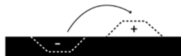
Fig.76.: The schematic drawing of dealing with the excess of dug out soil (Jančovičová, 2014)
